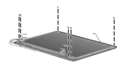
Where used: 6 screws that secure the display panel to the display enclosure
